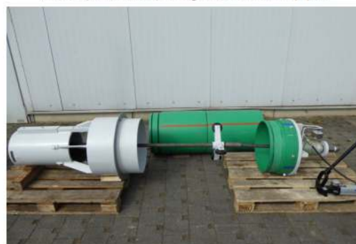
Hole Opener with pulling rods for HDPE pipes
