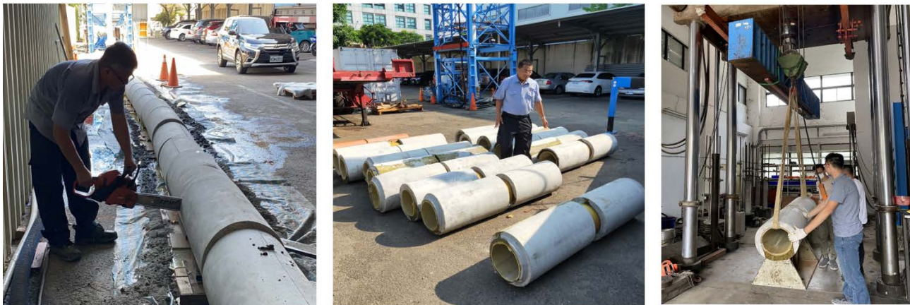
Cutting, transporting, testing of specimens.
