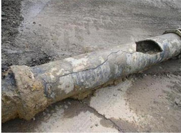
**Cast Iron Pipe Broken from Water Hammer**
