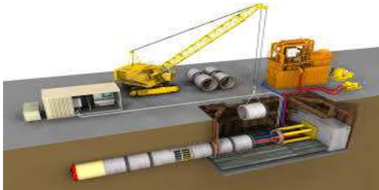
Micro tunneling - Pipe jacking > 400mm
