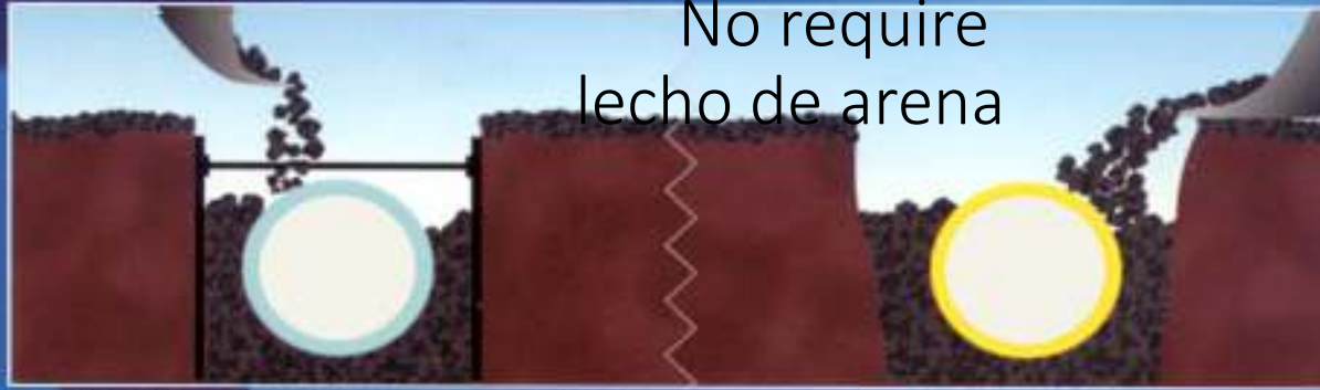
Open installation with reutilisation of excavated soil
