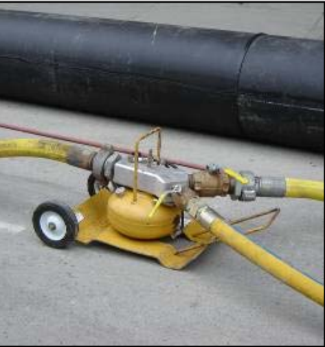
Oiler control station – supplies lubricated compressed air to activate pneumatic hammer
