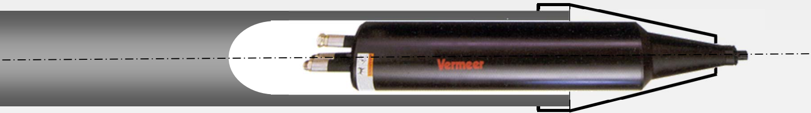
Assembled pneumatic tool with bursting head towing HDPE pipe
