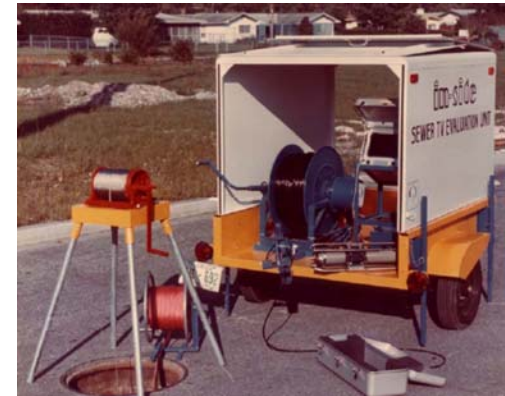
Hand winch skid mounted camera
