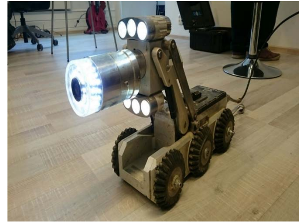
Automated sewer pipe inspection
