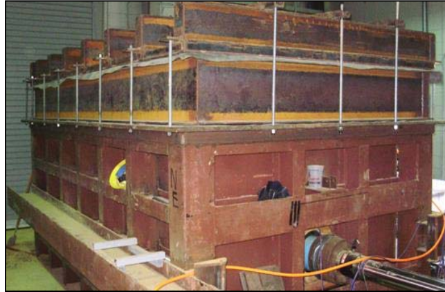
Soil box (small 12'x6'x6', large 10'x20'x11')
