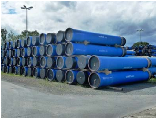
Fig. 4. Pipes with cement mortar coating (ZMU)
