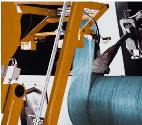
Fig. 2. Cement mortar application
