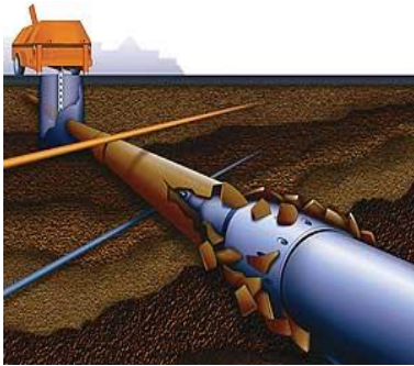
Figure 2. Pipe Bursting - How it works 1
