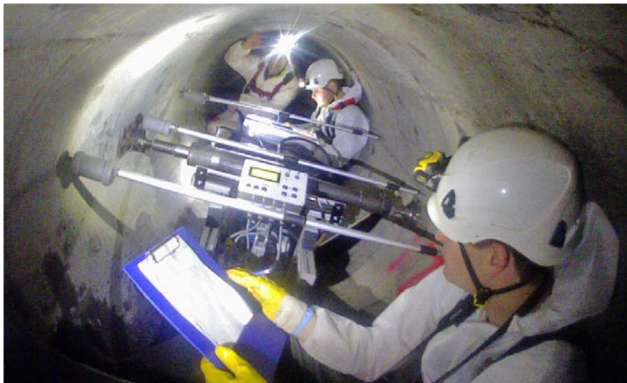
Figure 4. MAC test being carried out in the Braidley Tunnel.
