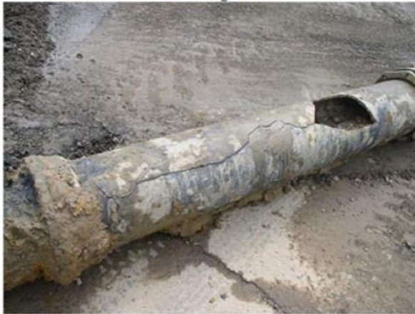
Cast Iron Pipe Broken from Water Hammer
