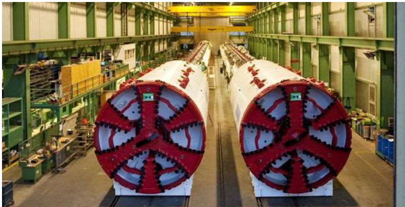
Figure 11 2 x EPB3600, OD 4390 in Herrenknecht factory, Schwanau, Germany
