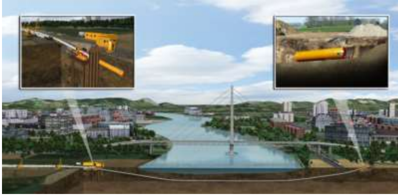
Figure 3 Schematic view of a Direct Pipe River crossing
