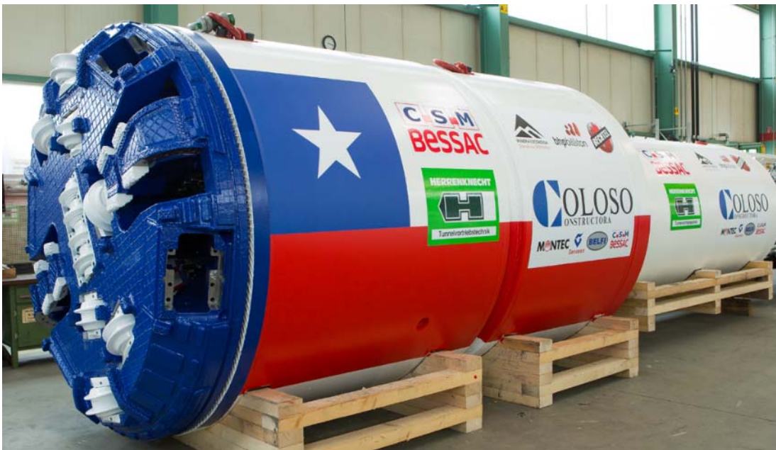
Figure 4. MTBM #1 before shipment
