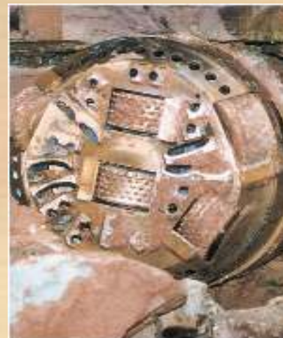
Cutting head design for use in soil and rock - Rock cutting head with insert roller cutters and small entry openings (F-ROK3)
