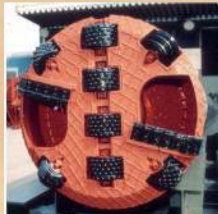
Cutting head design for use in soil and rock - Rock cutting head with disc and insert roller cutters (F-ROK2)
