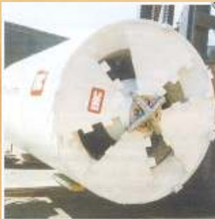
Cutting head design for use in soil and rock - Scraper cutting head with fixed soil entry openings (F-ICH)
