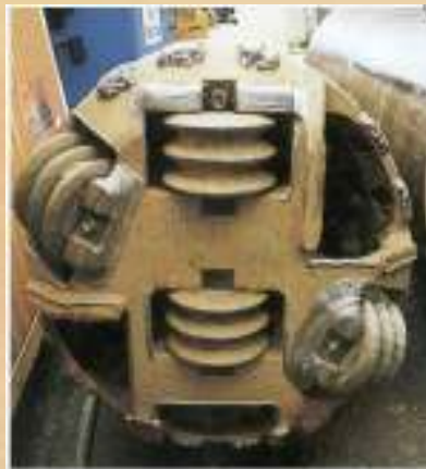
Microtunneling machine with hydraulic spot removal - Rock cutting head with disc cutters (F-Harot)
