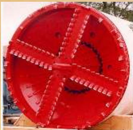
Microtunneling machine with hydraulic spot removal - Standard cutting head at the front of cutting wheel (F-WHITE)
